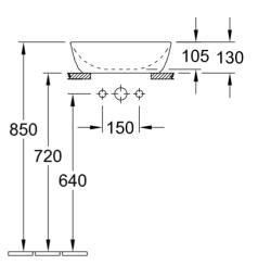
Note: All dimensions are in millimetres and are subject to normal manufacturing variations. Always use the physical product measurements for cut-outs and rough-ins as the technical details shown may differ from the actual product. Use acetic cured silicone sealant. Do not use epoxy type adhesives. Clean with damp cloth. Do not use abrasive cleaners, liquids or pastes.
