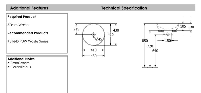
Note: All dimensions are in millimetres and are subject to normal manufacturing variations. Always use the physical product measurements for cut-outs and rough-ins as the technical details shown may differ from the actual product. Use acetic cured silicone sealant. Do not use epoxy type adhesives. Clean with damp cloth. Do not use abrasive cleaners, liquids or pastes.
