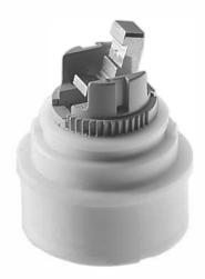
HANSAECO control cartridge 4.8; water brake at approx. 50% water rate; ceramic discs with integrated grease wells; scalding protection adjustable (except 0914, 0912, 0123, 0148); volume restrictor indefinitely variable up to approx. 6 l/min
