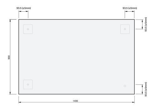
**IMPORTANT NOTE:** Throughout this guide, tolerance for mirror size may vary by ±1mm, tolerance for bracket position may vary by ±5mm. Please read the installation manual for detailed information on installing the product. St. Michel pursues a policy of continuing improvement in design and manufacturing of its products. The right is therefore reserved to vary specifications without notice.
